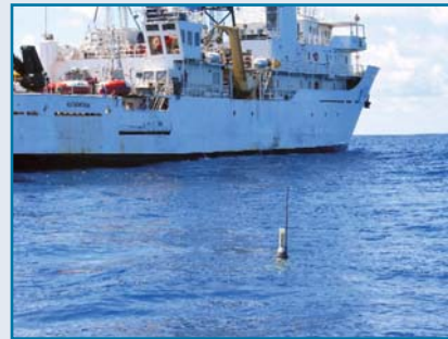
Deployment of an Argo profiling float from the NOAA Ship Ka'imimoana, tropical Pacific. These instruments measure temperature and salinity down to 2,000 meters.
